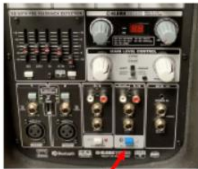
To connect, Push and hold the Blue Button. It will light up blue and “flash”
